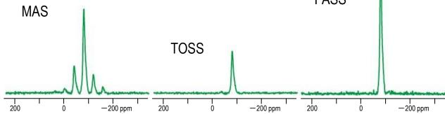
PASS spectra do not split the center peak into SSBs so that quantitative capability is guaranteed. Site fraction, for example, can be determined via lineshape analysis.
