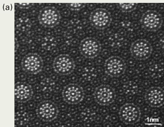
Fig. 3 (a) Atomic-resolution Z-contrast image of the decagonal quasicrystal  $\text{Al}_{70}\text{Mn}_{17}\text{Pd}_{13}$ , taken by the aberration-corrected 300 kV-STEM (R005 microscope equipped with the cold-field emission gun). (b) Calculated Z-contrast image based on the model structure proposed by x-ray analysis [10], revealing significantly different intensity distributions observed in (a). (c) Modified structure of the decagonal cluster and the corresponding simulated image.
