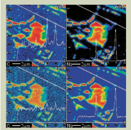
Fig. 6 WDS and EDS analysis of the area of view in Figure 5. Line profile of straight line in each map. Conditions: Accelerating voltage 7 kV; probe current 50 nA.
