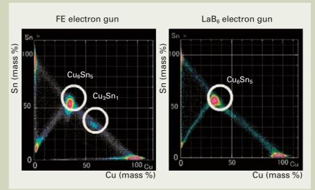
Fig. 14 Phase analysis of Cu-solder interface by FE and  $LaB_6$  guns. The FE gun was able to detect the presence of a  $Cu_3Sn_1$  alloy layer. See attached color images.
