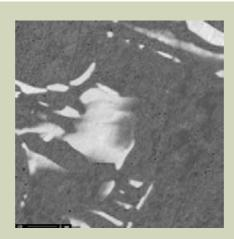
Fig. 5 BE composition image of stainless steel Numerous black particles  $0.1 \ \mu m$  or less present in matrix.
