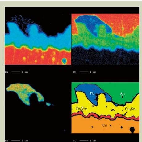
Fig. 13 X-ray image of the interface between solder and Cu. Cu<sub>6</sub>Sn<sub>5</sub> and Cu<sub>3</sub>Sn<sub>1</sub> alloys occur between the Sn and Cu. The image shows a Cu<sub>3</sub>Sn<sub>1</sub> alloy layer 0.2 μm thick. See attached color images. Conditions: Accelerating voltage 6 kV; probe current 10 nA.
