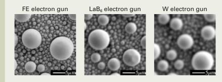
Fig. 3 Gold particles photographed with FE, LaB<sub>6</sub>, and tungsten guns. Conditions: Accelerating voltage 10 kV; probe current 100 nA.
